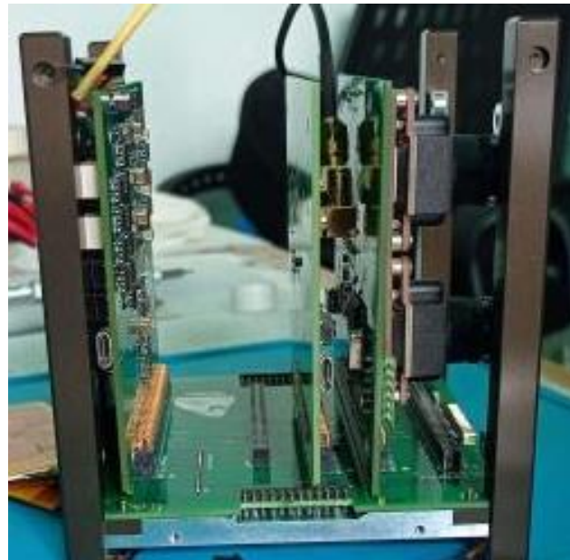
Boards placement on BPB
