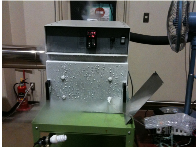
Fig. 43 Thermal cycle chamber at Kyutech
