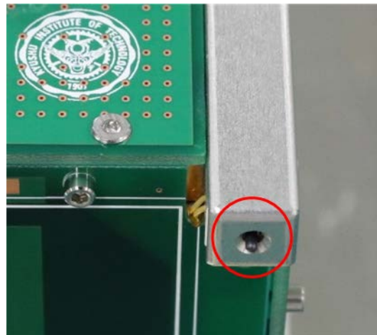
Fig. 10. Deployment switch (left) ©C&K; deployment switch in the rail (right)
