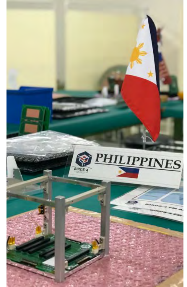
Backplane board and the structure of Maya-2, the Philippine's CubeSat (November 30)
