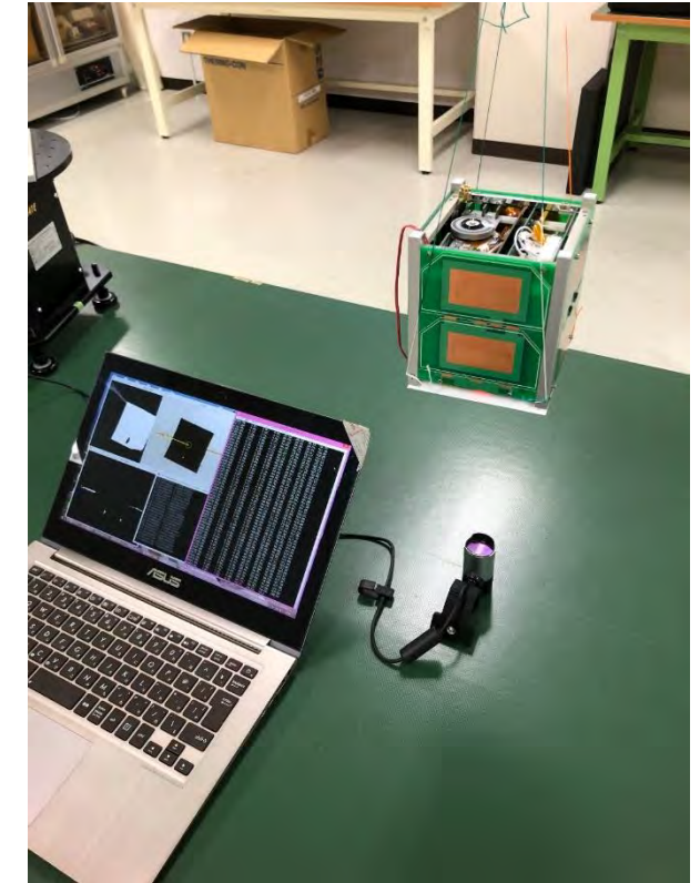
The satellite reaction result and testing set-up
