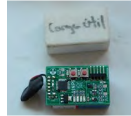
Before the competition begins, the organizers told all the teams that the cansat needed a payload dedicated space, but they didn't show how it looked like until the launch day (PCB down in the picture). The KurupiSat had a clever way to ensure that the space they had was correct. This way they got a better advantage of the available space (3D printed box on the top of the picture).
