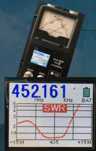
Measurement of the SWR of antenna
