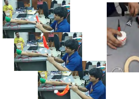
The team made some very important tests on the cansat, such as the parachute deployment mechanism they designed for the payload protection mission.
