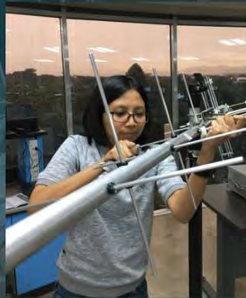
Placing the shaft retainers to lock the elements in place
