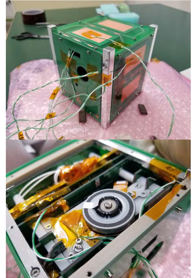
Thermocouples attached to the test article
