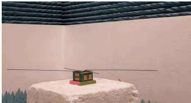
Antenna board inside the anechoic chamber
