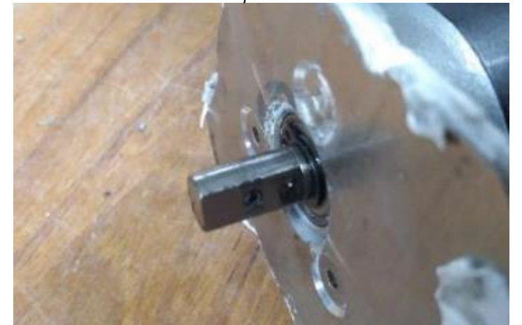
The motor shaft Some parts of the pin was damaged.
