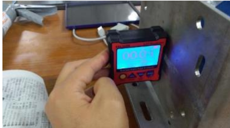
The calibration using the digital angle meter The rotator was connected at the controller and set 0 and 90 degrees. Based on the calibration, the controller converts the pulse from the rotary encoder into an angle.
