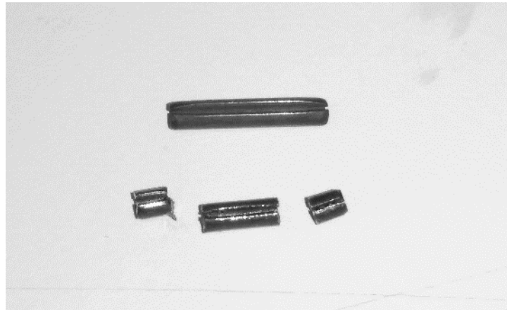
The new pin (upper) and the broken pin(lower) The gear and motor of rotator is protected from this.
