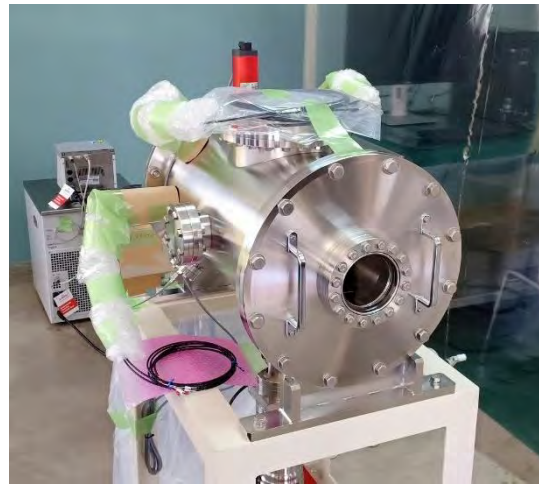
Thermal vacuum chamber for unit testing
