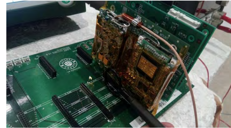
Boards under test: FAB, OBC/EPS board and COM board
