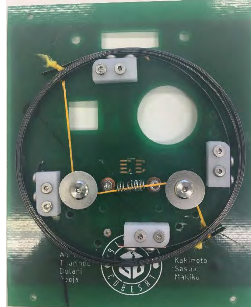
Before the antenna deployment
