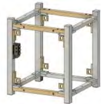
Modified structure of BIRDS-4 to be used as Hentenna
