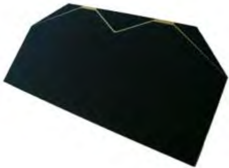
Triple junction solar cell being used in BIRDS project [Image source]
