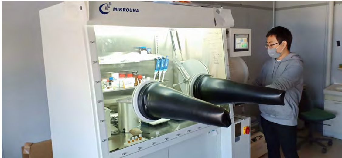
Shuzhang preparing for Perovskite cell fabrication inside glow box
