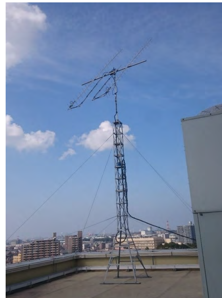
New BIRDS GS Yagi antenna on rooftop
