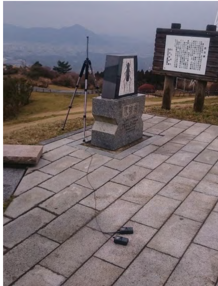
Hand held radio and dipole antenna with stand originally used as tripod for camera. I made parts for fixing the antenna with a 3D printer.
