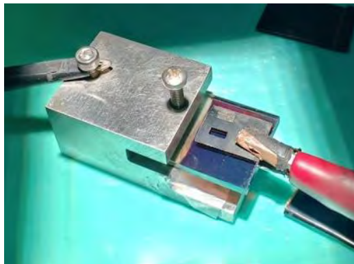
Testing the Perovskite solar cells under solar simulator.
