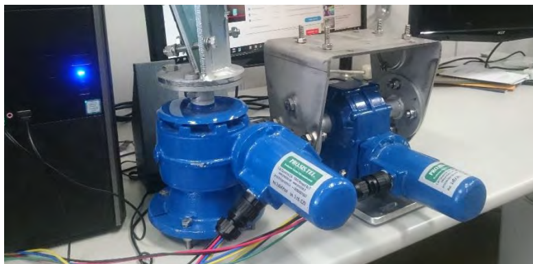
New BIRDS rotator - left for azimuth, right for elevation
