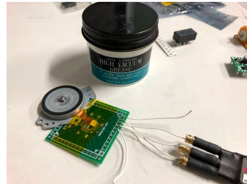
CD drive spindle motor to be used as a reaction wheel
