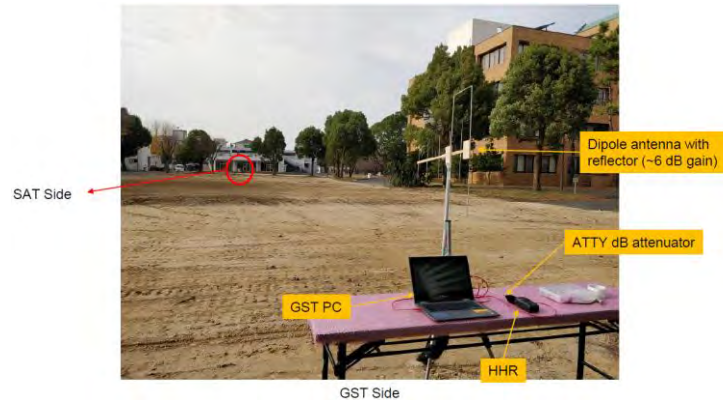
Setup at the ground sensor terminal side
