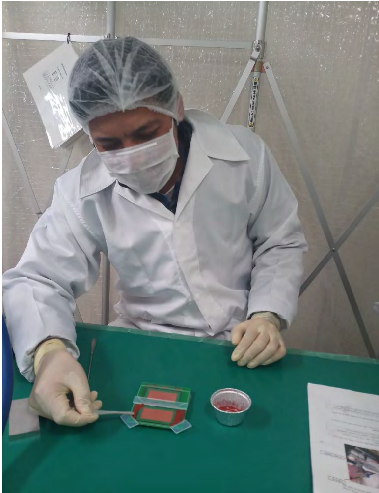
Hari applying RTV for solar cell attachment on the PCB.
