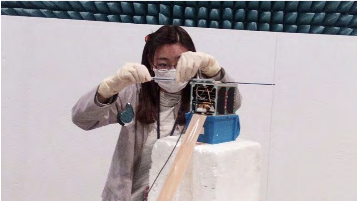
Measuring antenna length
