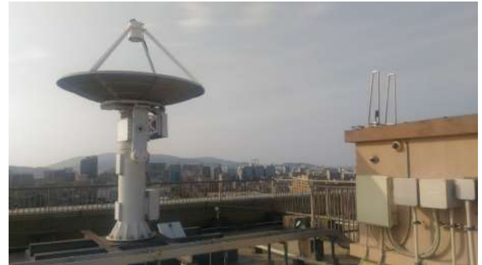
HORYU-IV S-band Dish Antenna
