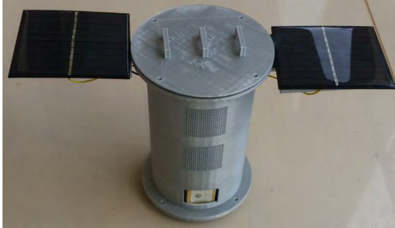
CanSat_Rwa; Can-sized satellite in Rwanda, can be used as an educational tool of space technology
