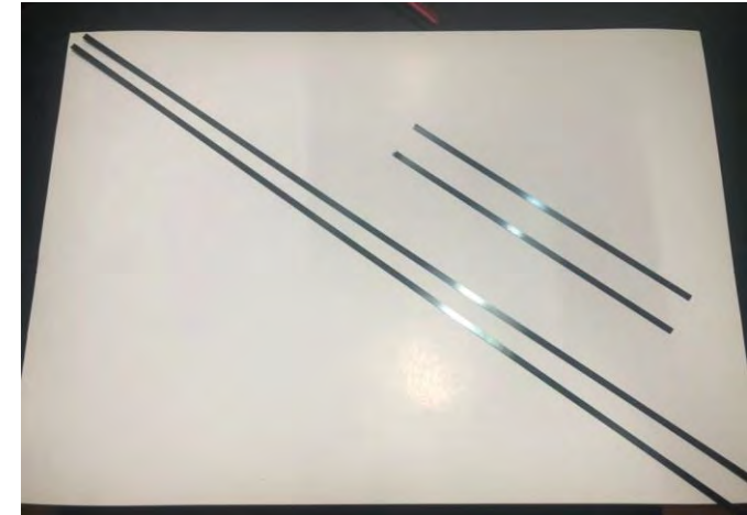
Figure 5: The steels that were cut into specific length as dipole antenna.
