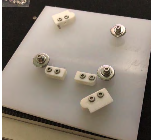
Figure 4: Additional three (3) screws or washers were used as anchor points on the mock-up board.
