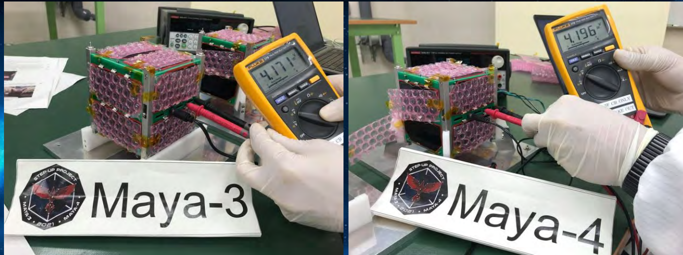
Measuring the battery voltage of Maya-3 and Maya-4 prior to ending the charging procedure
