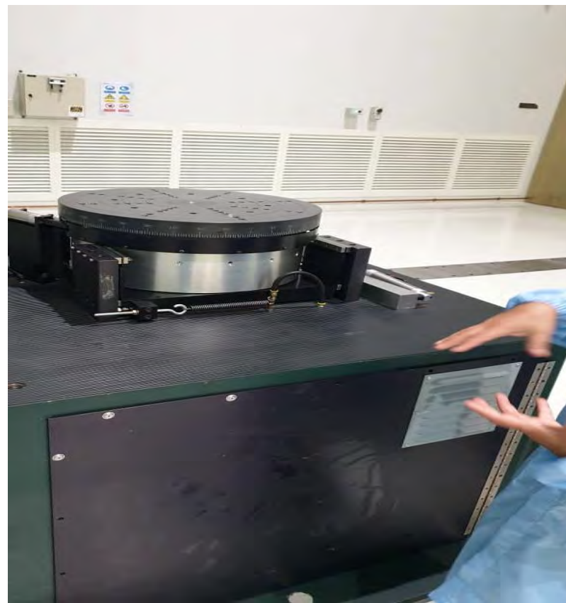
Figures 8: MYSA's AIT facility also has Centre of Gravity machine that can be utilized for structure balancing test.
