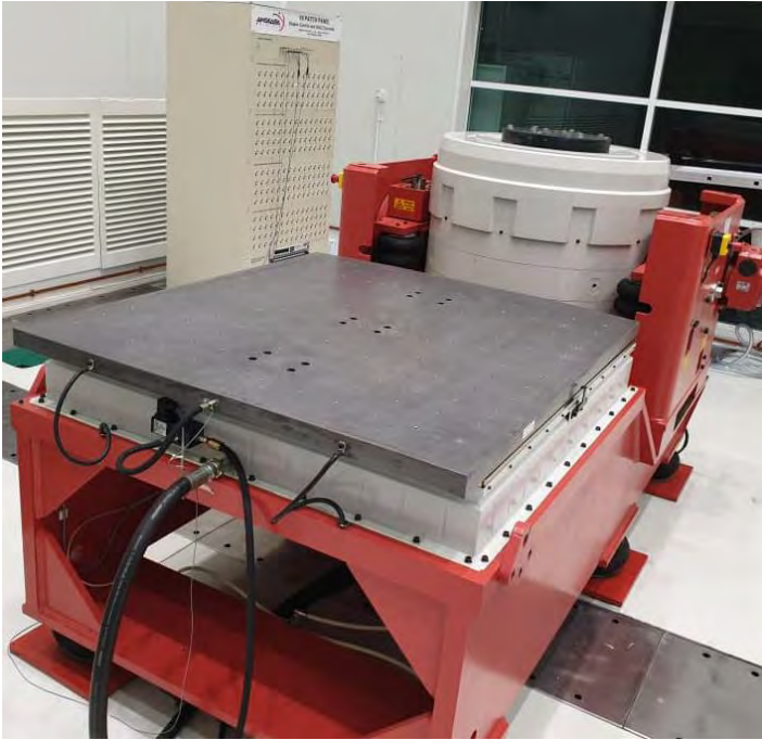
Figures 4: Shaker machine for vibration test in MYSA. The facility is equipped with data acquisition (DAQ) system and compatible software for various types of vibration test such as modal survey, random vibration, sine burst, and quasi static.
