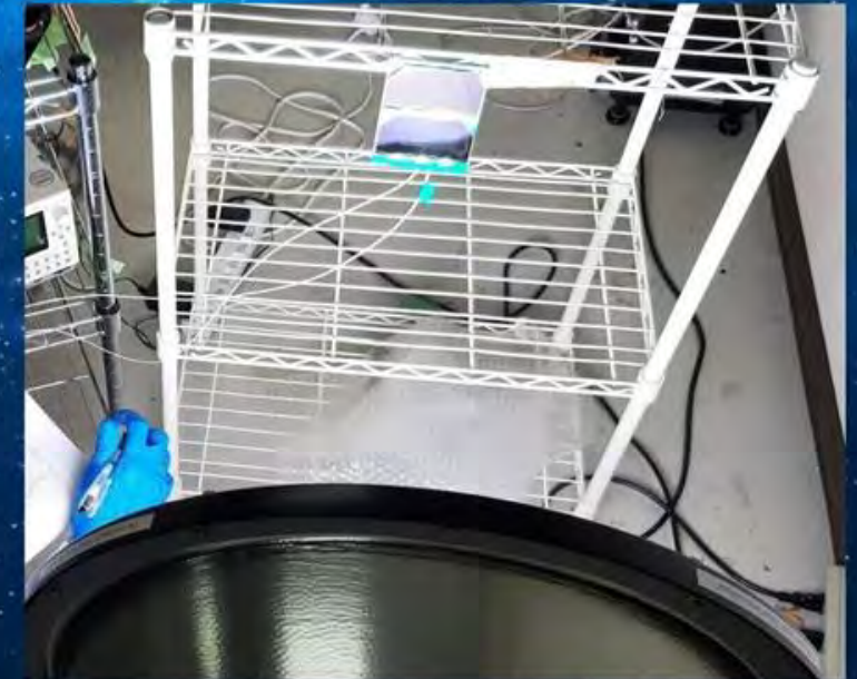
Testing and characterization of solar panel boards using a solar simulator at KyuTech
