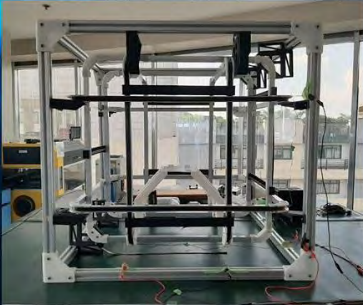
Helmholtz cage at the ULyS 3 ES used for characterizing the magnetometer
