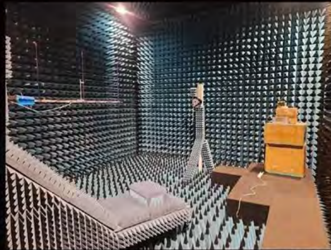
Sensitivity test setup in the Full Anechoic Chamber (FAC)
