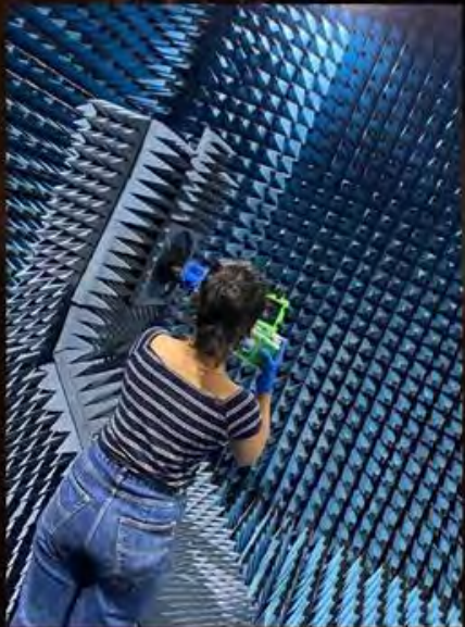
Val strapping in the cubesat onto the L-Bracket for radiation pattern measurement
