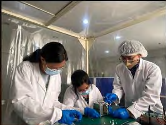
Comms team assembling the CubeSat for radiation pattern measurement
