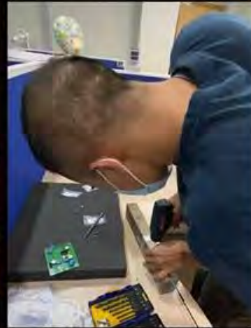
Jim attempting to drill mount holes onto antenna material
