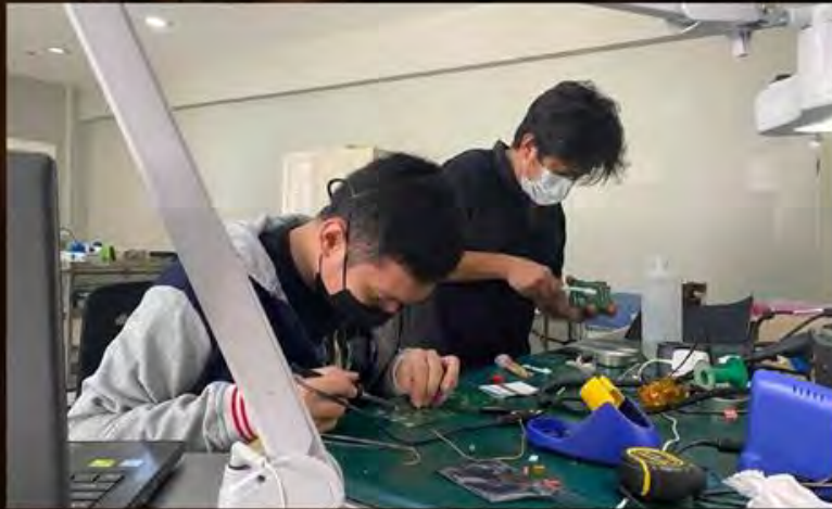
Gio (left) soldering components on the -Y panel for testing, Ronald (right) preparing the BPB for testing
