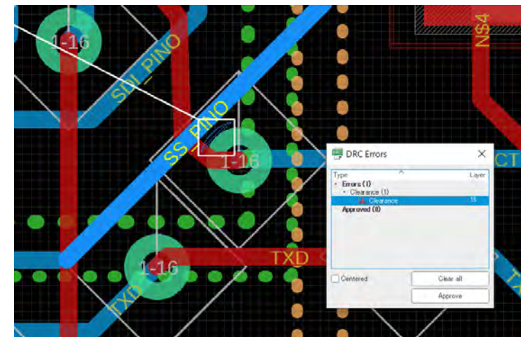
DRC detects the clearance problem
