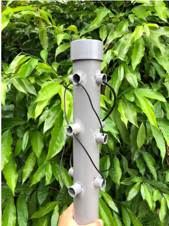
QFH Antenna Structure
