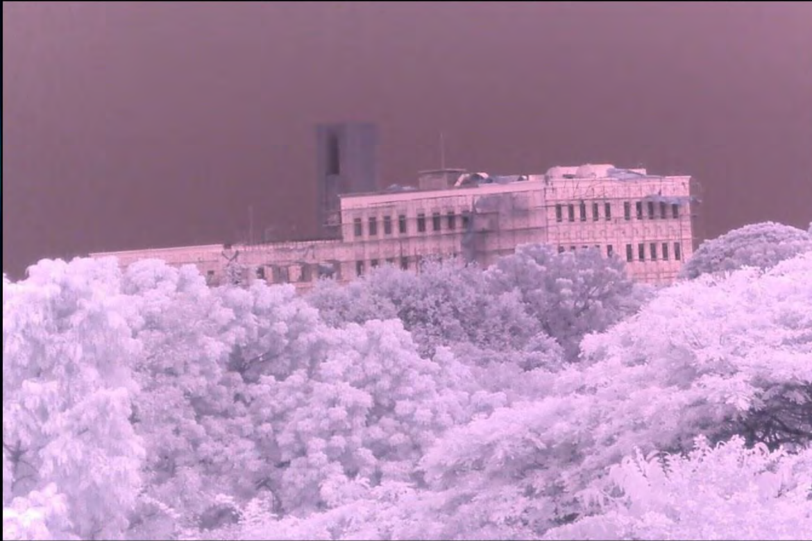
NIR image of a building about 800m away from the OV5642 camera. The camera lens has a focal length of 25mm.
