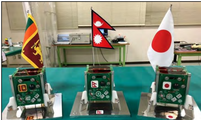
BIRDS 3 satellites ( showing the –X panel board)
