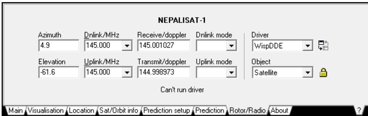
At “Rotor/Radio”, you can control your ground station antenna via driver.
