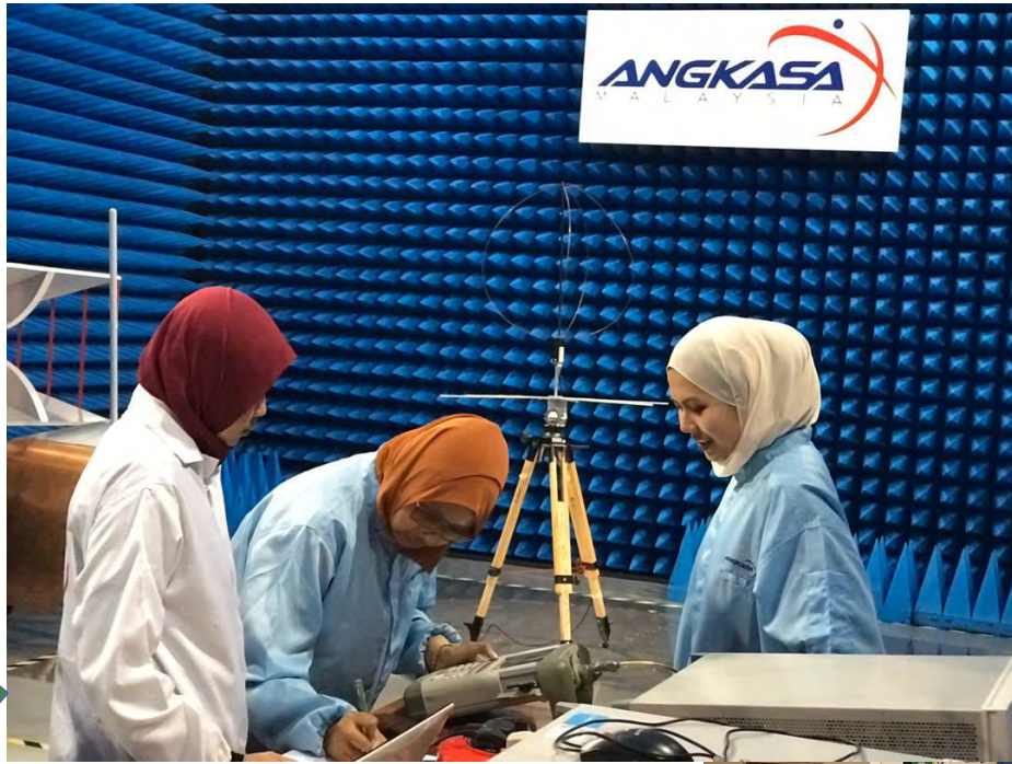
Fig. 4: One of the facilities provided by MYSA, anechoic chamber for antenna measurement
