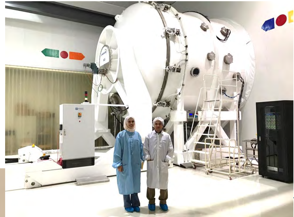
Fig. 5: One of the facilities provided by MYSA, TVT chamber for satellite testing
