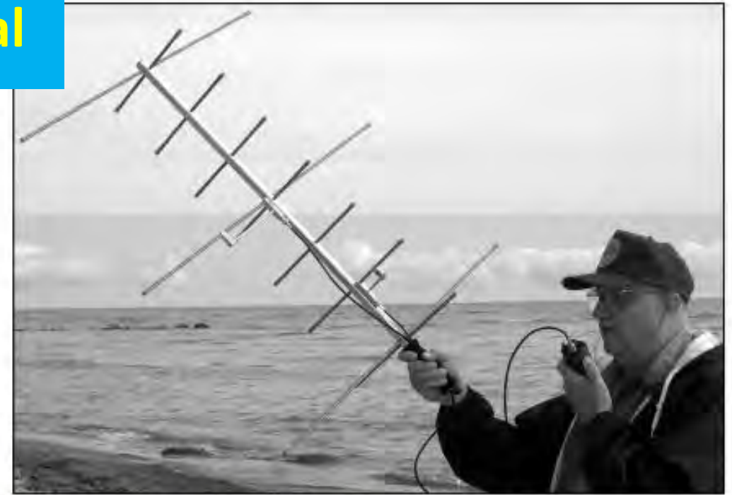
The author uses a Kenwood TH-78A dual-band HT and a lightweight Arrow Antenna to make a contact through AO-51 from the shores of Lake Huron in Michigan. When used with a 5 watt, full-duplex handheld in an open location free of foliage, such as a beach or a field, the antenna provides enough uplink and downlink gain to successfully work the FM birds, even on passes close to the horizon. (KB1OGF Photo)
