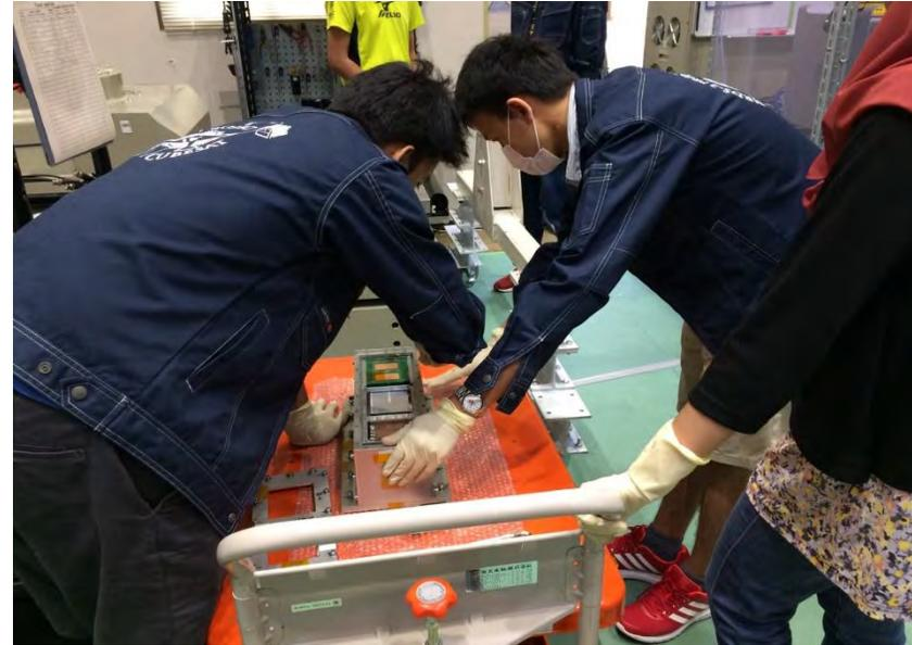
*Fig. 3: EM inserted and fixing into the POD*
