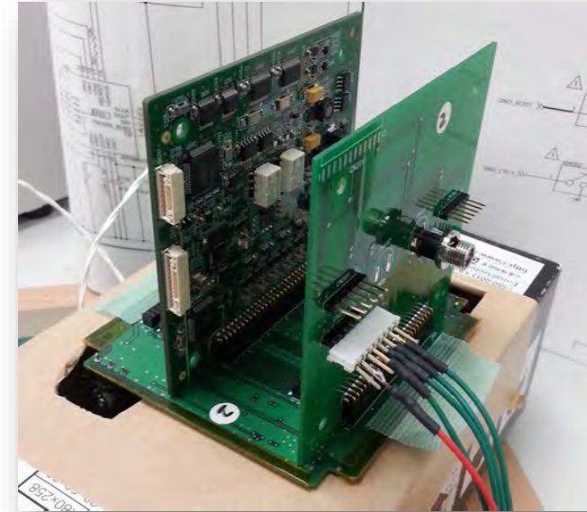
PCB (Printed Circuit Board) of OBC, EPS and COM ( Manufactured by Sagami Tsushin Co., Ltd )
