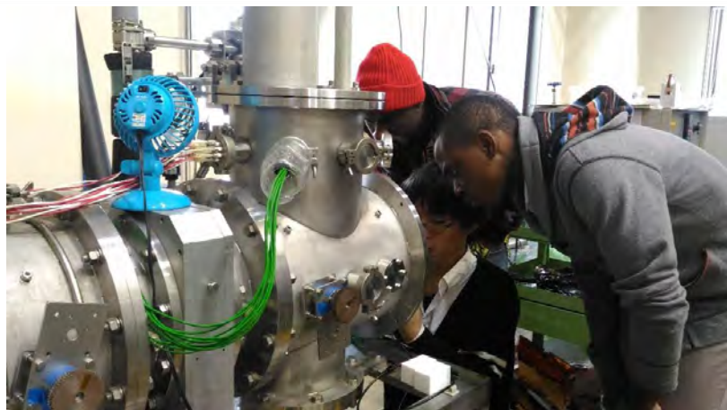
Setting our boards into thermal vacuum chamber. Photo taken by Apiwat
