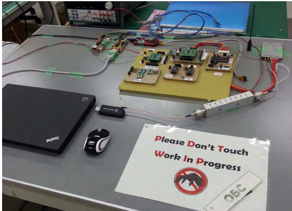
BBM board in the OBC work area
